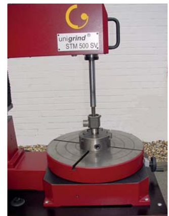
Grinding safety relief valve on rotary table
