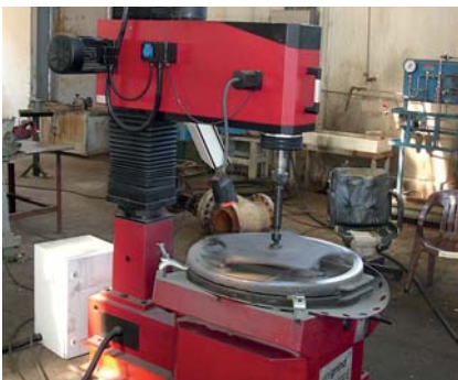
STM 800 E Grinding of gate valve wedge
