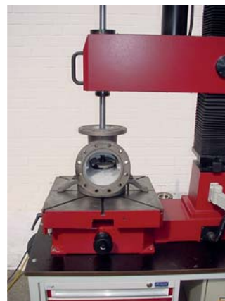
Grinding gate valve on tilting table
