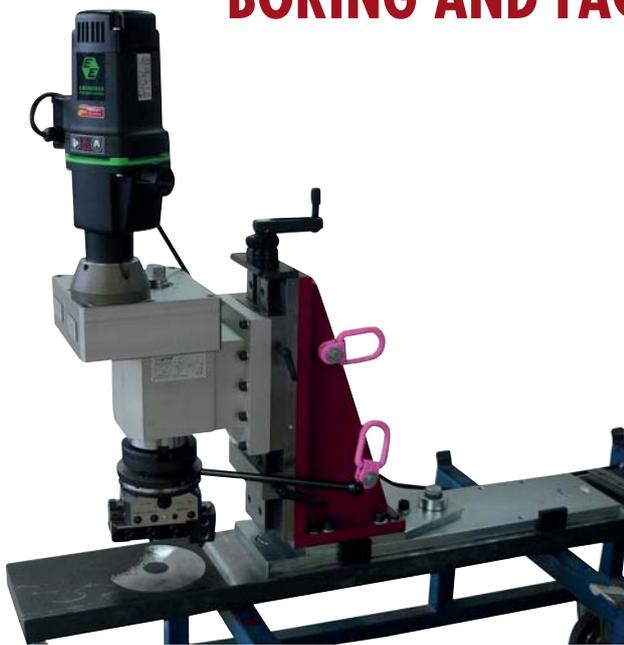
Mobile boring and turning machine for all boring and turning operations during steel work.
