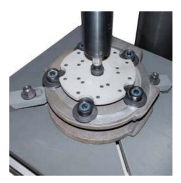
Grinding of gate valve wedge
