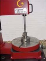
Grinding gate valve on tilting table
