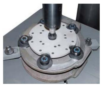
Grinding gate valve wedge with planet grinding disk
