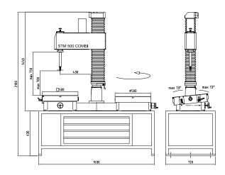
Stationary valve grinding and lapping machine for sealing surfaces in gate, globe, check valves, gate valve wedges and safety relief valves.
