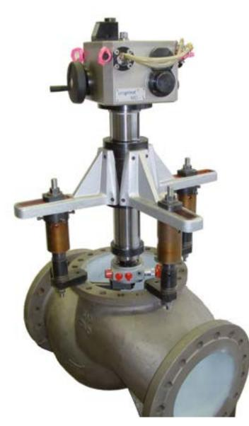
MD 1 Machining of globe valve seat
