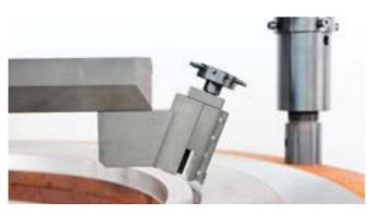
FDA 1200, RTJ 'V' grooves machining
