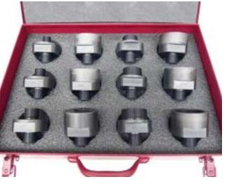
thread adapters for values with NPT and BSP thread
