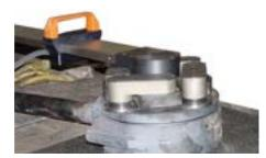
SHS 600 grinding of gate valve wedge
