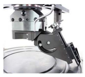
FDA 500, RTJ 'V' grooves machining
