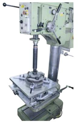
UNT 2 + Adapter, Grinding gate valve wedge
